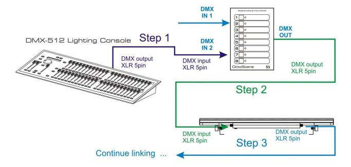
2. Then connect from the OctoScene's output to the input of the following fixture as stated above and continue the linking until last planned fixture is conected in your DMX signal data chain.
