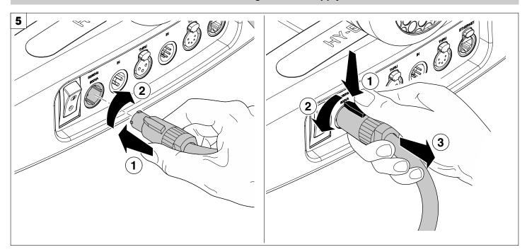
Connecting and disconnecting power cable - Fig. 5
