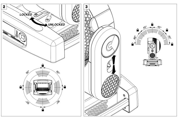
PAN Mechanism Lock and Release (every 90°) - Fig. 2
